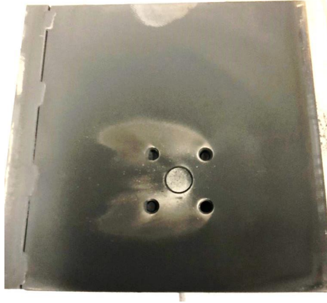
Figure 6.13 – Post-exposure image of the ET target holder with a SiC sample, uncleaned. The ET plasma jet impacted this holder at about 45^\circ from right to left, which generated the deposition pattern around the sample and the surrounding empty holes.
